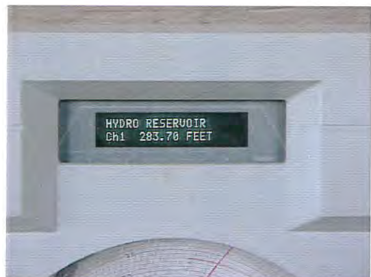
Gainer Dam reservoir elevation monitoring equipment
