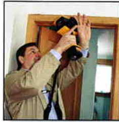
Thermographic scan to reveal poor or missing insulation
