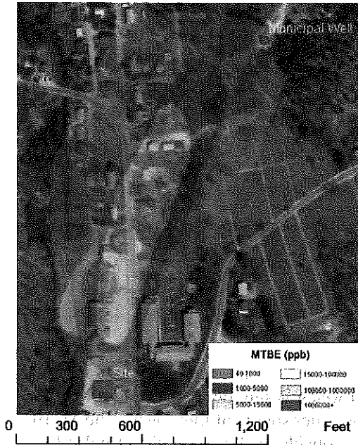
Figure 1: Currently known extent of the Pascoag MTBE plume in the bedrock aquifer.
