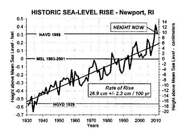
Difference between mean sea level at Newport, R.I., from 1983 to 2001 and mean annual sea level plotted for each year between 1930 and 2012. The blue trend line shows a 8.7 inch rise through 2012, which is equalto a 10.6 inch (26.9 cm) increase in sea level per century. GRAPH COURTESY OF JON BOOTHROYD, 2012.
