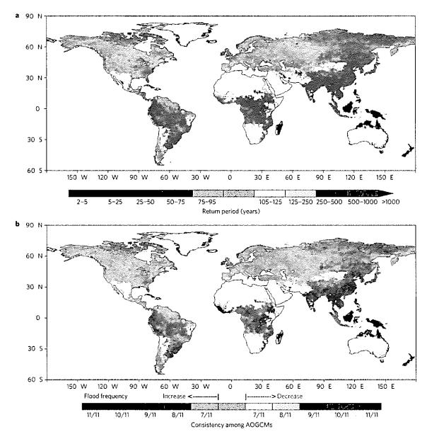
Figure 1 Projected change in flood frequency. a, Multi-model median return period (years) in 21C for discharge corresponding to the 20C 100-year flood. b, Model consistency. Grid cells with mean annual discharge of a retrospective simulation<sup>13</sup> for 1979-2010 of <0.01 mm d<sup>-1</sup> are screened out. The case for the RCP8.5 scenario is shown.
