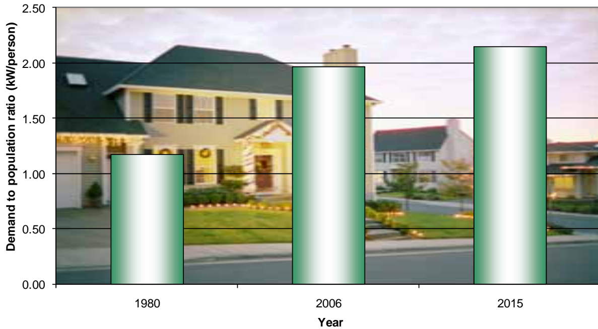
Figure 3-2. The ratio of peak electricity demand to population is expected to rise from around 1.2 kW in 1980 to 2.2 kW in 2015, (data source ISO-NE).
