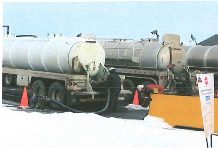
Oilfield waste arrives by tanker truck at a wastewater disposal facility near Platteville, Colo. After removal of solids and oil, the wastewater is injected into a deep well for permanent storage underground. Photo by Bill Ellsworth, USGS.
