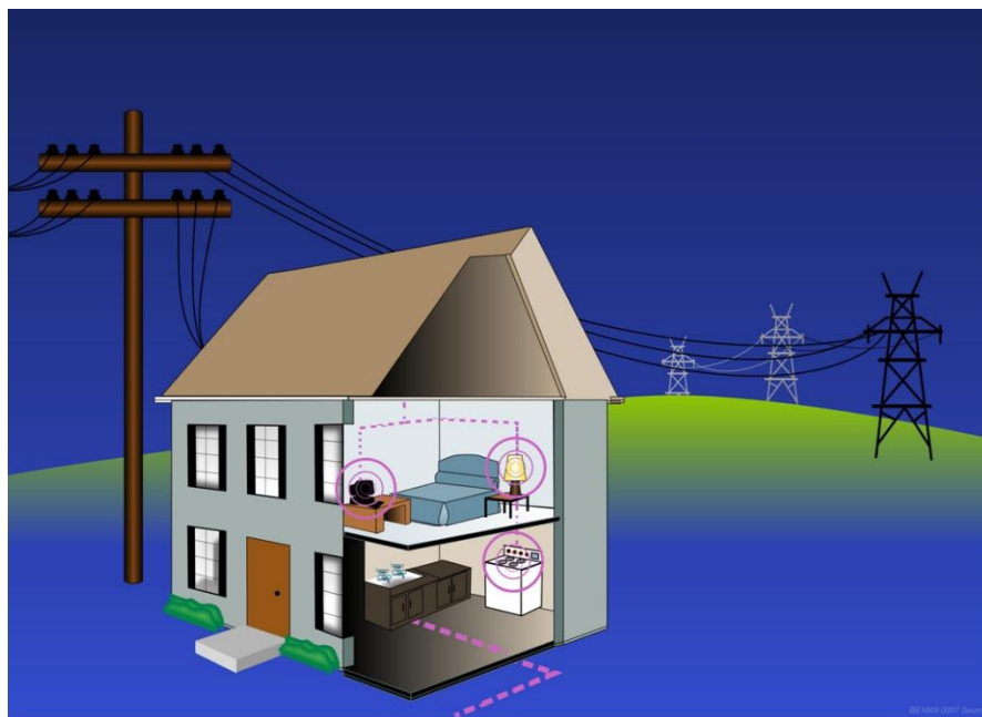
Figure 1. Common sources of ELF EMF in the home (appliances, wiring, currents running on water pipes, and nearby distribution and transmission lines).
